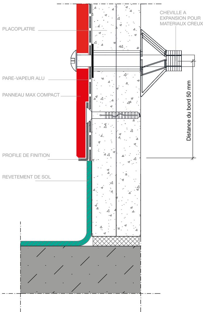
COUPE VERTICALE D'UN RACCORD AU SOL ANTICHOC AVEC UN REVÈTEMENT DE SOL EN PVC
