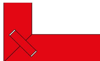
ASSEMBLAGE D'ANGLE AVEC LANGUETTE
