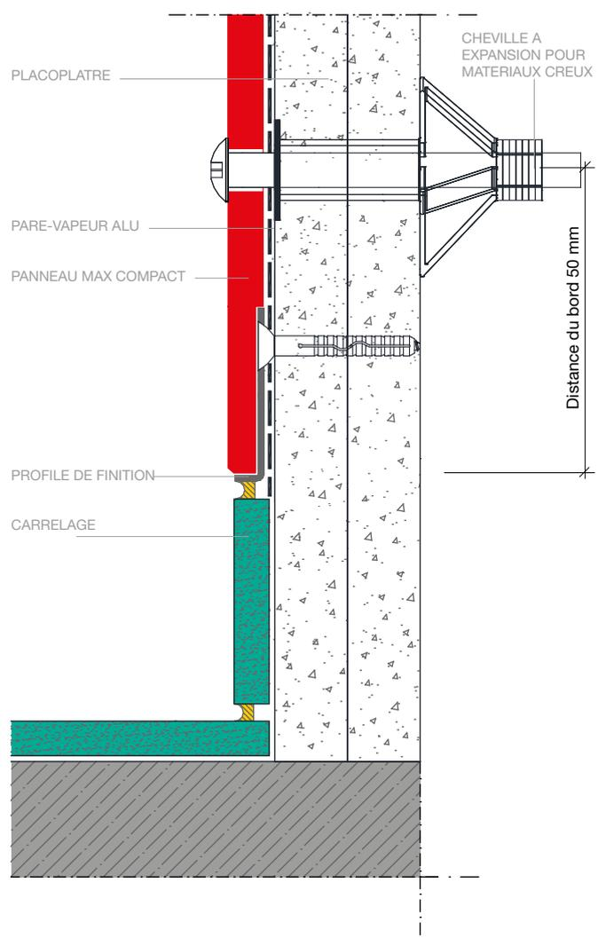
FIG. 1 COUPE VERTICALE D'UN RACCORD AU SOL ANTICHOC EN AFFLEUREMENT AVEC LE CARRELAGE
