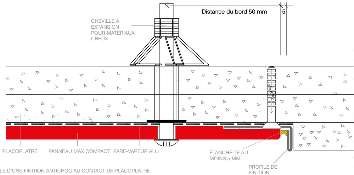
COUPE VERTICALE D'UNE FINITION ANTICHOCC AU CONTACT DE PLACOPLATRE
