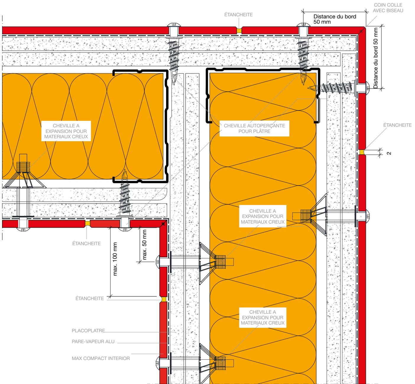
COUPE HORIZONTALE DE LA STRUCTURE DE COIN, AVEC COINS INTERIEUR ET EXTERIEUR ASSEMBLES EN ONGLET
