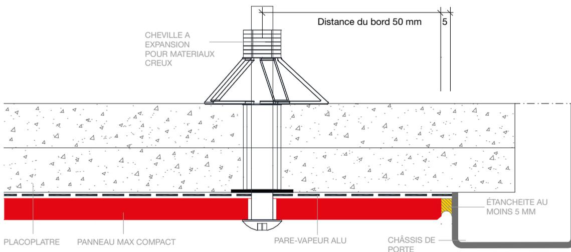
COUPE VERTICALE D'UNE FINITION ANTICHOCC AU CONTACT DU CHÂSSIS DE PORTE
