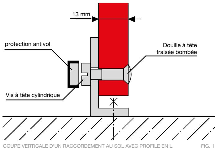
COUPE VERTICALE D'UN RACCORDEMENT AU SOL AVEC PROFILE EN L FIG. 1
